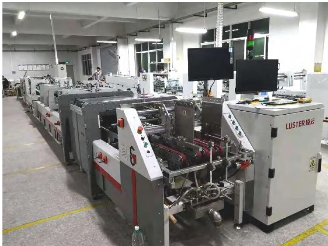
Automatci Gluing machine with on-line quality inspection device
